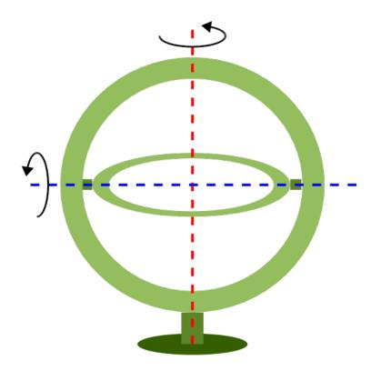
In the image above, the outer-gimbal axis, or sweep-angle axis, is the N/S axis (y) while the inner-gimbal axis, or fixed-angle axis, is the E/W axis (x).
