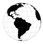
The geos projection pictures how a geostationary satellite scans the earth at regular scanning angle intervals.
