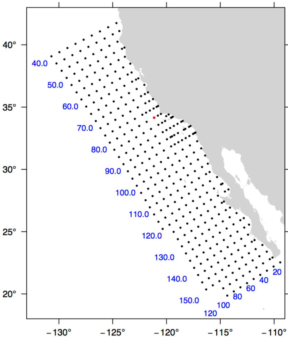
The coordinate system is based on the Mercator projection with units rotated -30 degrees from the meridian so that they are oriented with the coastline of the Southern California Bight and Baja California. Lines increase from Northwest to Southeast. A unit of line is 12 nautical miles. Stations increase from inshore to offshore. A unit of station is equal
