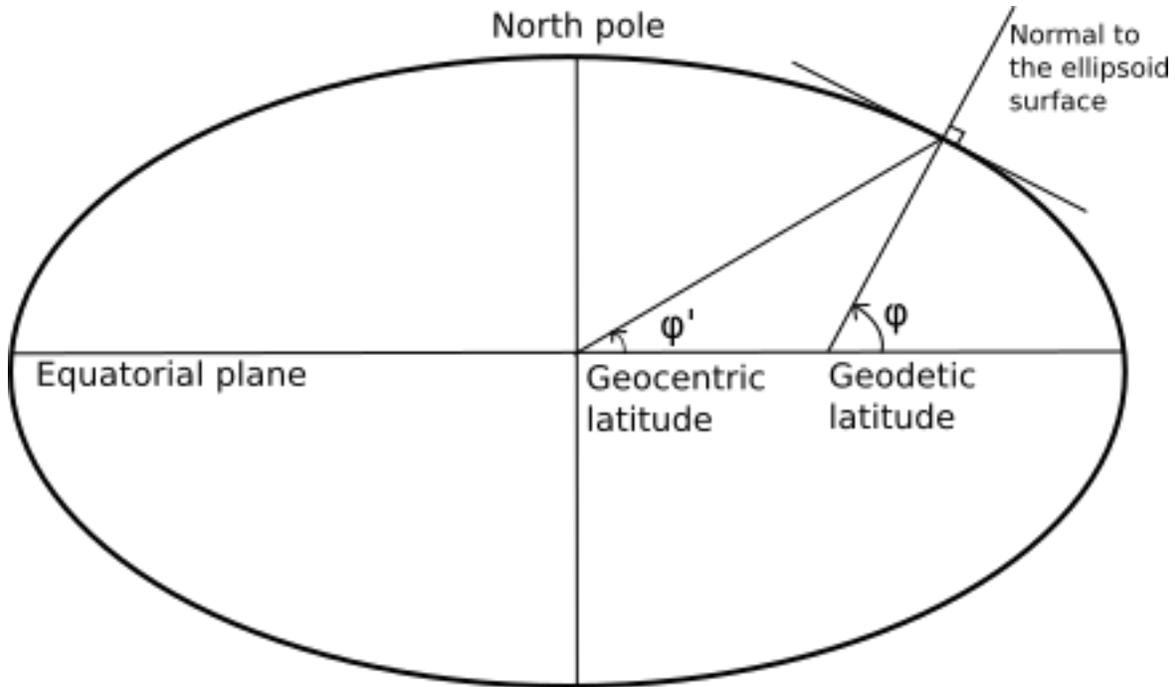
**Note:** This conversion must be distinguished from the *Geodetic to cartesian conversion* which converts geodetic coordinates to geocentric coordinates in the cartesian domain.
