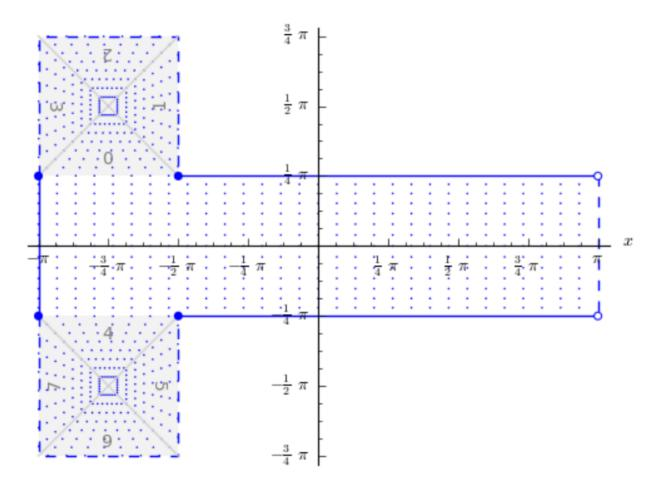
rHEALPix is a projection based on the HEALPix projection. The implementation of rHEALPix uses the HEALPix projection. The rHEALPix combines the peaks of the HEALPix into a square. The square's position can be translated and rotated across the x-axis which is a novel approach for the rHEALPix projection. The initial intention of using rHEALPix in the Spatial Computation Engine Science Collaboration Environment (SCENZGrid).
