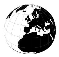
Tilted Perspective is similar to *Near-sided perspective* (nsper) in that it simulates a perspective view from a height. Where nsper projects onto a plane tangent to the surface, Tilted Perspective orients the plane towards the direction of the view. Thus, extra parameters specifying azimuth and tilt are required beyond *nsper* ''s h. As with nsper, lat\_0 & lon\_0 are also required for satellite position.
