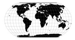
The Natural Earth projection is intended for making world maps. A distinguishing trait is its slightly rounded corners fashioned to emulate the spherical shape of Earth. The meridians (except for the central meridian) bend acutely inward as they approach the pole lines, giving the projection a hint of three-dimensionality. This bending also suggests that
