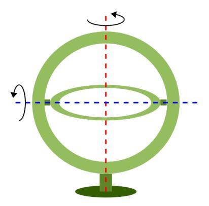
In the image above, the outer-gimbal axis, or sweep-angle axis, is the N/S axis (y) while the inner-gimbal axis, or fixed-angle axis, is the E/W axis (x).
